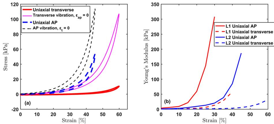
Fig. 2. (Color online) (a) The stress-strain curves obtained from uniaxial and biaxial tests for L2. (b) The derived tangent Young's moduli derived from the uniaxial tests for larynges L1 and L2.
