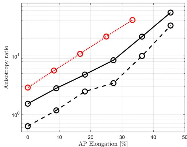
Fig. 4. (Color online) The stiffness anisotropy ratio, calculated as the ratio between the AP and transverse tangent Young’s moduli, as a function of AP vocal fold elongation. Solid line: L2. The dotted and dashed line are an underestimation of the anisotropy ratio for L1 and L2, respectively.
