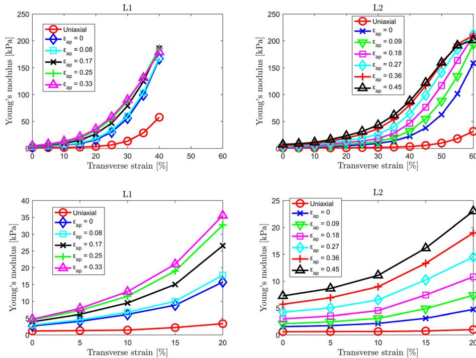
Fig. 3. (Color online) The transverse tangent Young’s modulus as a function of the transverse strain for different conditions of AP elongation. The bottom panels show the same data but for a smaller range of transverse strain that is more likely to occur in normal phonation.
