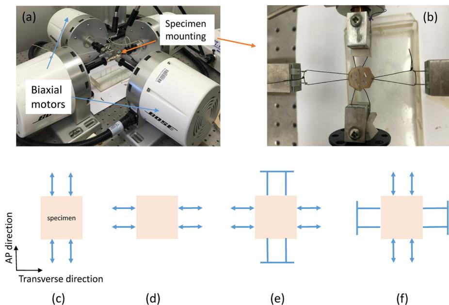
Fig. 1. (Color online) The experimental setup for the biaxial tests (a) and tissue mounting (b). (c)–(f) show the four experimental protocols used in this study, including two uniaxial settings and two biaxial settings.
