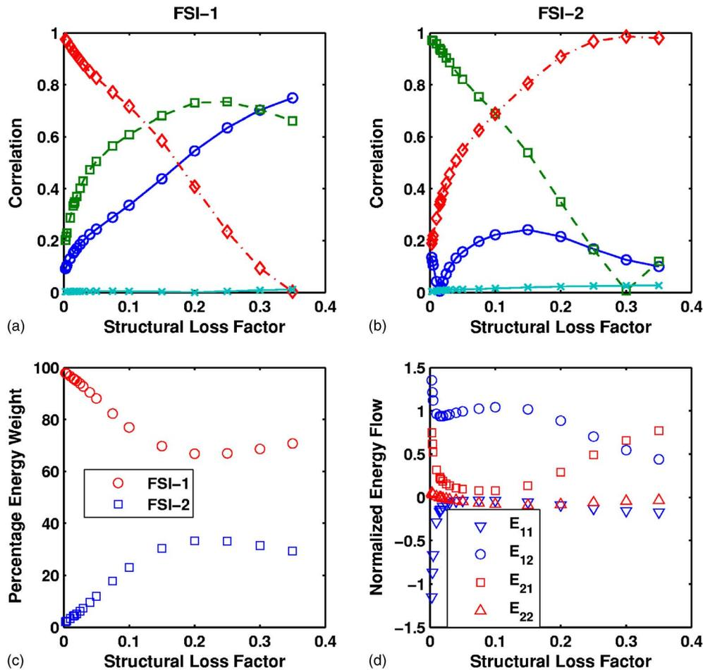
FIG. 13. (Color online) Correlation between the FSI-1 mode (a) and FSI-2 mode (b) and the first four *in vacuo* eigenmodes ( $\circ$ : first;  $\square$ : second;  $\diamond$ : third;  $\times$ : fourth *in vacuo* eigenmodes), relative energy weights of the two FSI modes (c), and normalized contributions to the total energy flow by individual interaction terms (d) as a function of the structural loss factor. Model parameters were given in Eq. (28),  $Q = Q_2\dot{q} + Q_1\dot{q} + Q_0q$ .
