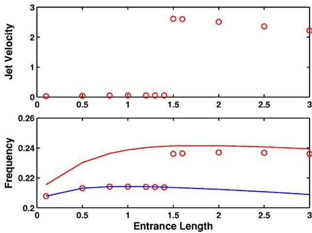
FIG. 12. (Color online) Onset jet velocity (top) and frequency (bottom) as a function of the length of the entrance section  $T_{\text{inf}}$ , for model parameters given in Eq. (28),  $Q = Q_2\dot{q} + Q_1\dot{q} + Q_0q$  for  $\sigma=0$ . The two solid lines indicate the second and third *in vacuo* eigenfrequencies.
