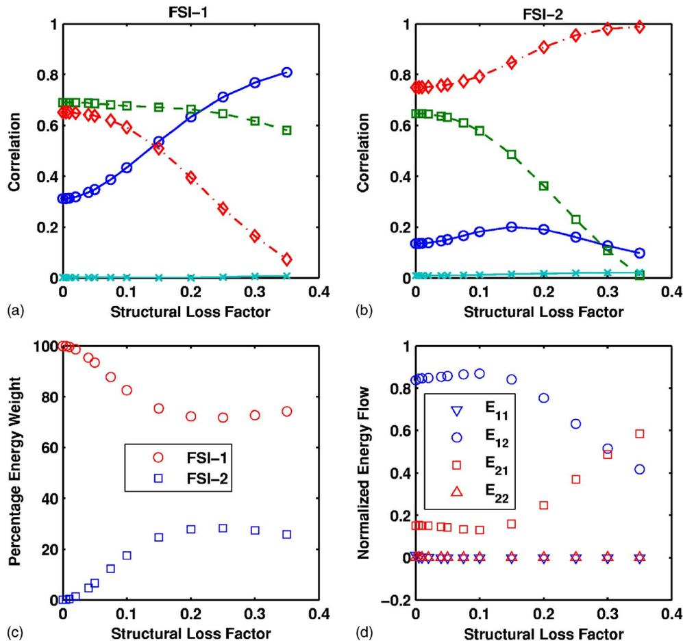
FIG. 9. (Color online) Correlation between the FSI-1 mode (a) and FSI-2 mode (b) and the first four *in vacuo* eigenmodes ( $\circ$ : first;  $\square$ : second;  $\diamond$ : third;  $\times$ : fourth *in vacuo* eigenmodes), relative energy weights of the two FSI modes (c) and normalized contributions to the total energy flow by individual interaction terms (d) as a function of the structural loss factor. Model parameters were given in Eq. (28),  $Q=Q_0q$ .
