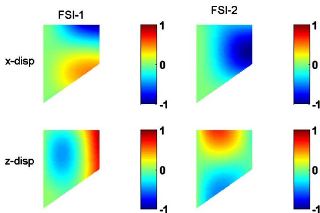
FIG. 6. (Color online) Vibration patterns of the FSI-1 (left) and FSI-2 (right) modes at onset for case shown in Fig. 5(a) ( $Q=Q_0q$ , model parameters given by Eq. (28),  $\sigma=0$ ). The first and second rows show the  $x$  component (medial-lateral direction) and  $z$  component (inferior-superior direction) of the eigenmodes, respectively.
