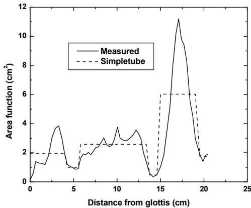
**Fig. 4. Measured area function and simple-tube area function.**
